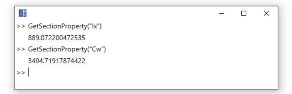
b. The maximum or minimum values for the various stresses and the warping function can obtained directly using the command line.
