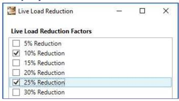
In VA 17 you specify one or more levels for reducing live loads in the Load Case Manager. his feature uses the building code combination feature to generate additional load combinations, one set for each level you enable. You can then associate a Design Group with one of these levels to take advantage of the reduced demands. Easy and no "black box" voodoo!
