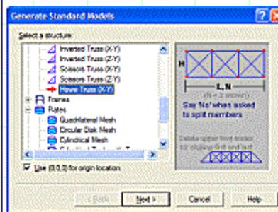
Feel free create more parametric model definitions to help you speed up your work. You could generate a full 3D Howe Truss including all the lateral bracing, floor beams and stringers all in one step if you have just a little 'programmer' in you.
